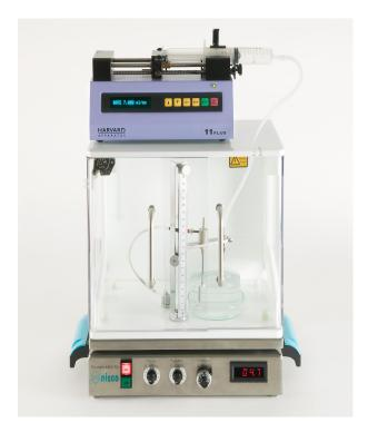
The method is based on using an electrostatic potential to pull droplets from a needle top into a gelling bath. A voltage is applied between the needle feeding the alginate solution and an electro conductive solution underneath.
